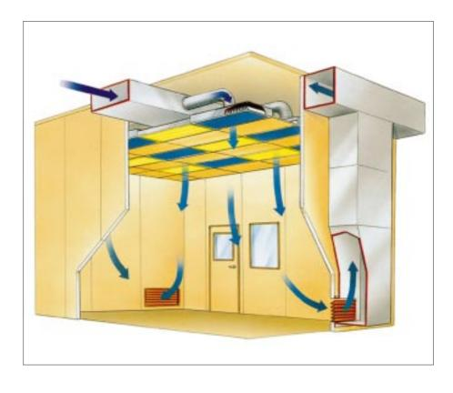
In a non-laminar cleanroom or, to use its official name, non-unidirectional airflow cleanroom, air enters the room via filters in the ceiling, and is exhausted via grilles in the wall close to the floor.
