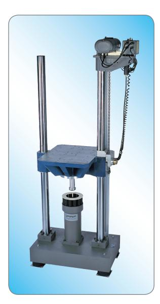
The Model 65/81 Shock Test System provides the pulse quality and system reliability needed for testing small to mid-size products. The Model 65/81 meets or exceeds many industrial, military, and corporate shock testing standards and specifications.
