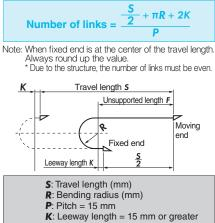
\* Set the leeway length K to 23 mm or greater for support roller arrangement Set the installation distance of support rollers to 350 mm or less.
