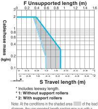
Vote: A the Conductors in the shaded area and on the load diagram, the unsupported length section may run with a sag. This may cause interference between the cable carrier and equipment depending on the installation conditions. Contact a Tsubaki representative for further information.
