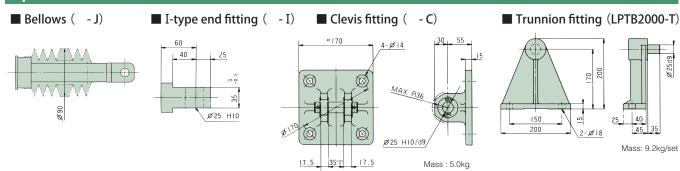
Note) Shipped as attached to the main body. The XA dimensions are the same as the standard U-type end fitting. Note) Shipped attached to the main body. If it needs to be shipped individually, consult us.
