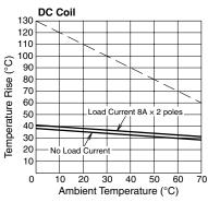
The above temperature rise curves show characteristics when 100% the rated coil voltage is applied. The slanted dashed line indicates allowable temperature rise for the coil at different ambient temperatures.
