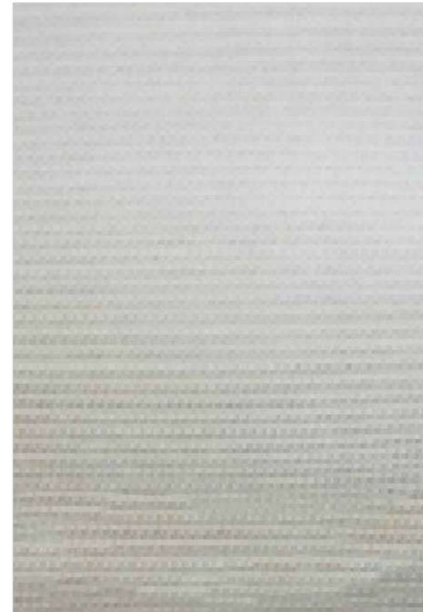
Glass fiber felt 800g with ptfе membrane
