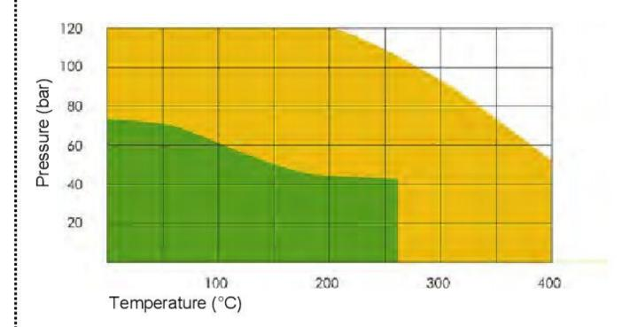
The P x T diagram above indicates the service limits for **NA -1100** considering the simultaneous influence of pressure and temperature (chemical suitability assumed). The green area represents the normal service limits, while the orange coloured area shows the maximum application limits. For those cases, please consult our technical department.
